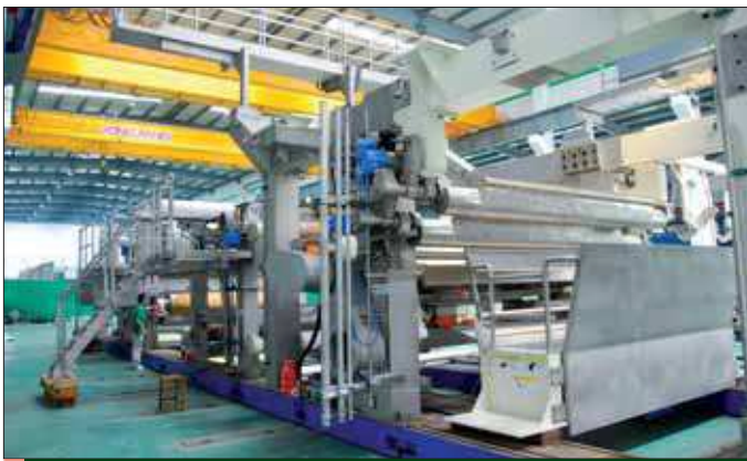
Wet end section of Intelli-Tissue™ 900 during pre-assembly Intelli-Tissue™ 900 型紙機濕部正在進行預安裝
